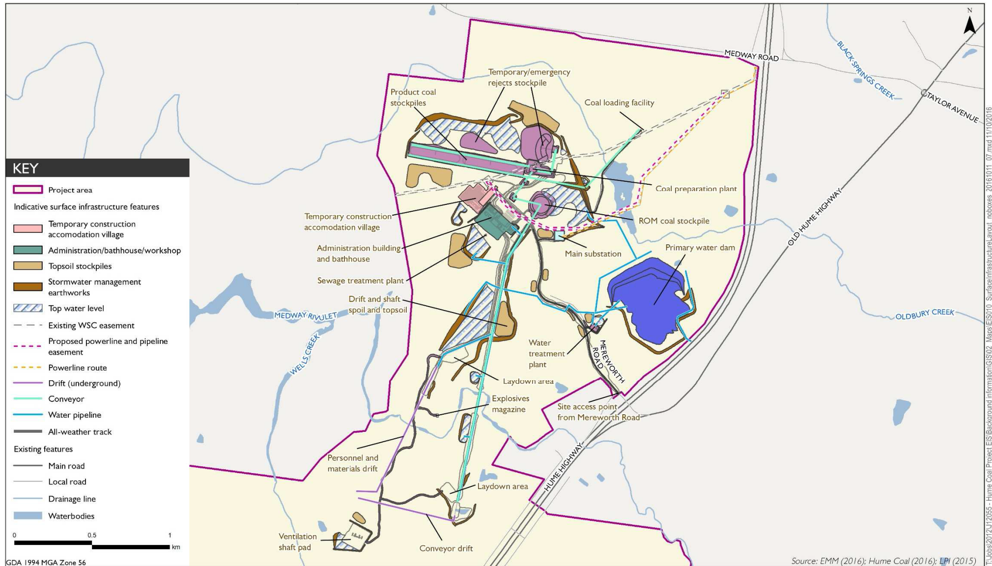
Figure 1.3. Indicative surface infrastructure layout.
