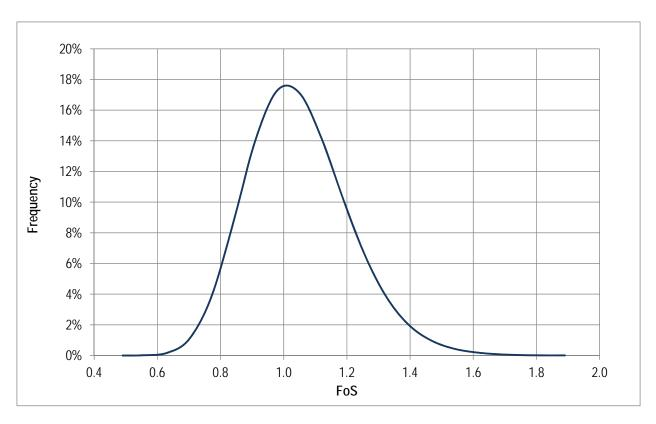
Figure 2. Distribution of pillar FoS of 1.0 using the UNSW pillar strength formula
