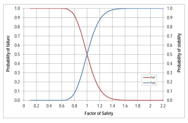
Figure 3. Probabilities of failure and stability associated with the UNSW pillar strength formula
