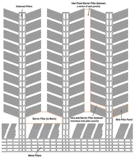
Figure 1. Illustration of the proposed layout showing the different coal pillar types (after Mine Advice, 2017)
