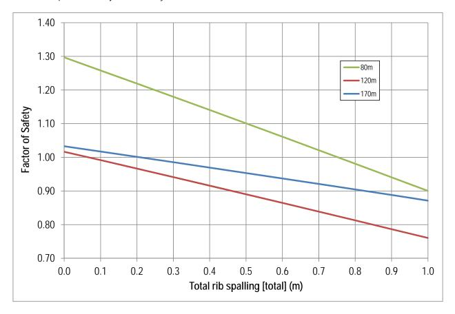
Figure 4. Pillar FoS reduction due to pillar spalling
