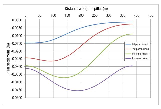
Figure 21. Surface subsidence at 170m depth following the extraction of four panels
