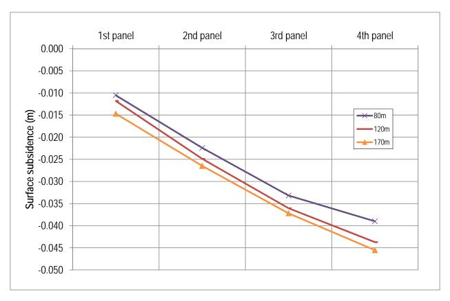
Figure 23. Comparison of maximum surface subsidence at 80m, 120m and 170m depth following the extraction of the panels
