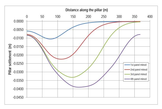
Figure 19. Surface subsidence at 80m depth following the extraction of four panels
