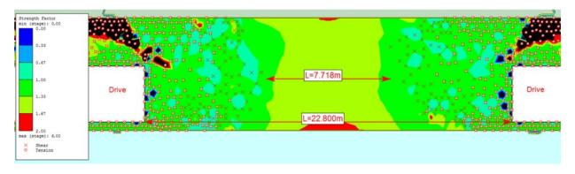
Figure 25. Strength factor of the intra-web pillar in the case of complete failure of web pillars
