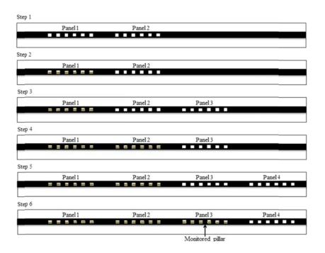
Figure 14. Excavation and backfilling sequence
