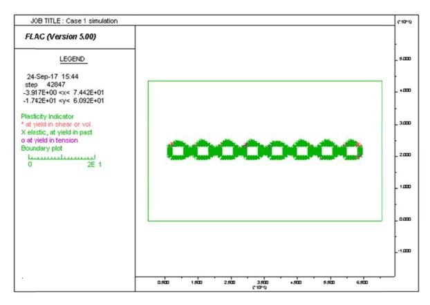
Figure 10. Plastic indicator in Case 1
