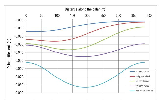
Figure 24. Surface subsidence in worse case, i.e. all web pillars have failed with no remnenat
