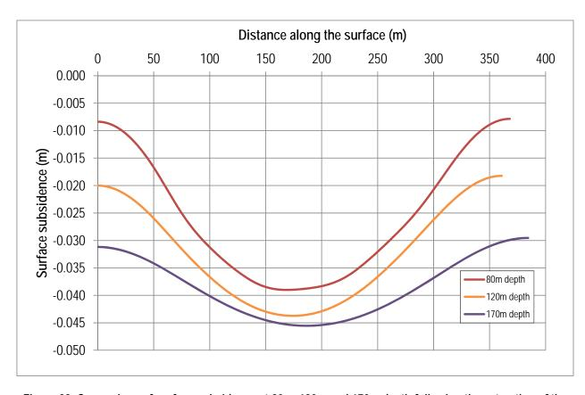
Figure 22. Comparison of surface subsidence at 80m, 120m and 170m depth following the extraction of the four panels
