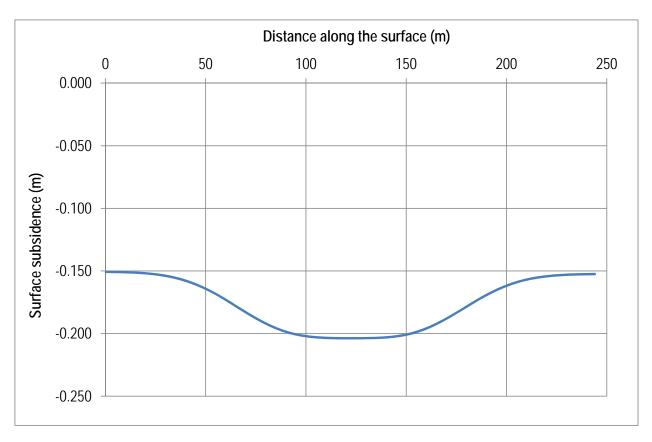
Figure 18. Surface subsidence due to settlement of inelastic pillars
