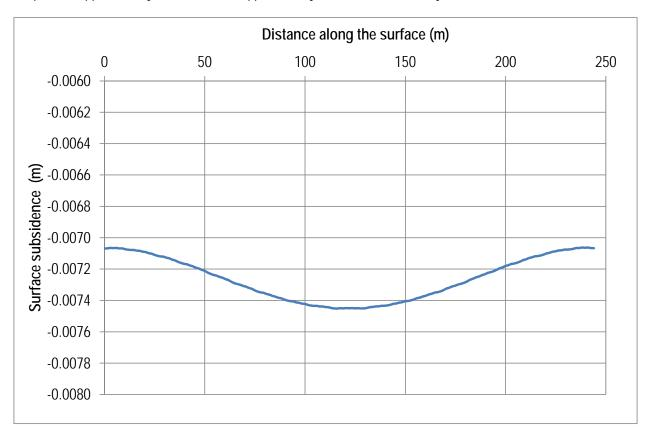
Figure 17. Elastic settlement of an elastic pillars on surface
