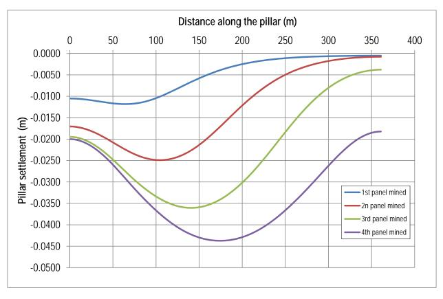
Figure 20. Surface subsidence at 120m depth following the extraction of four panels
