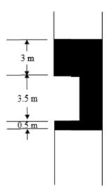
Figure 8. Geometry of coal pillar model with 3 m coal roof and 0.5 m floor
