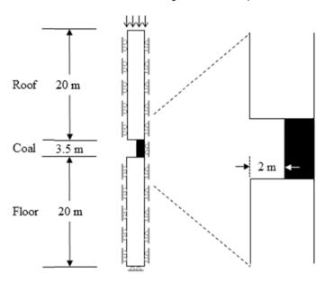
Figure 6. Geometry of coal pillar model
