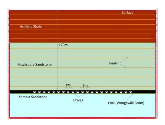
Figure 16. Phase2 layout to assess the elastic settlent of we pillars
