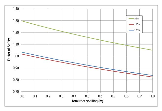
Figure 5. Pillar FoS reduction due to roof spalling
