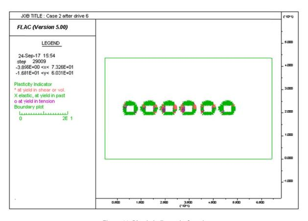
Figure 11. Plastic indicator in Case 2
