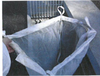
Figure 5-11 A typical Enviropod pit insert assembly (Source: Stormwater360)
