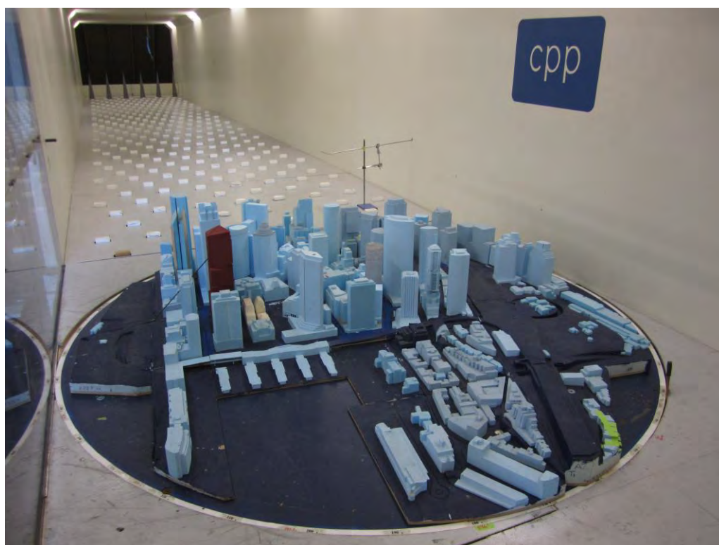
Figure 5: Existing Goldfield House model in the wind tunnel viewed from the north – Configuration B
