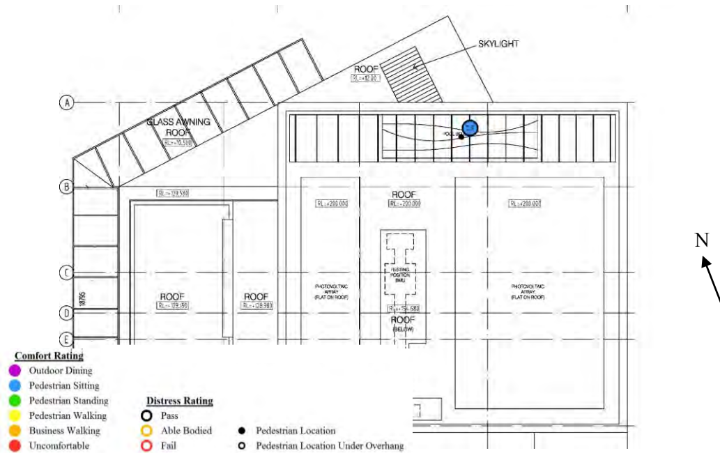
Figure 13: Pedestrian wind speed measurement locations with comfort/distress ratings – Configuration A Tower A Roof
