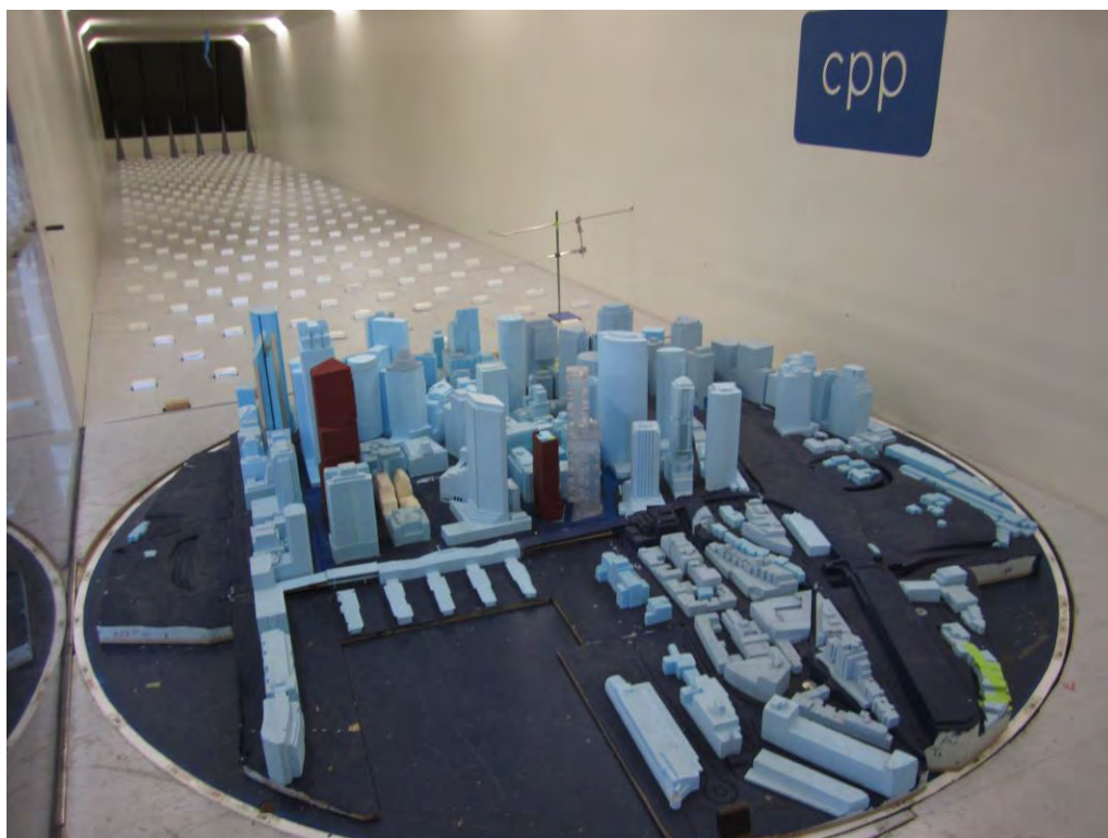
Figure 4: Proposed Sydney 1 model in the wind tunnel viewed from the north – Configuration A
