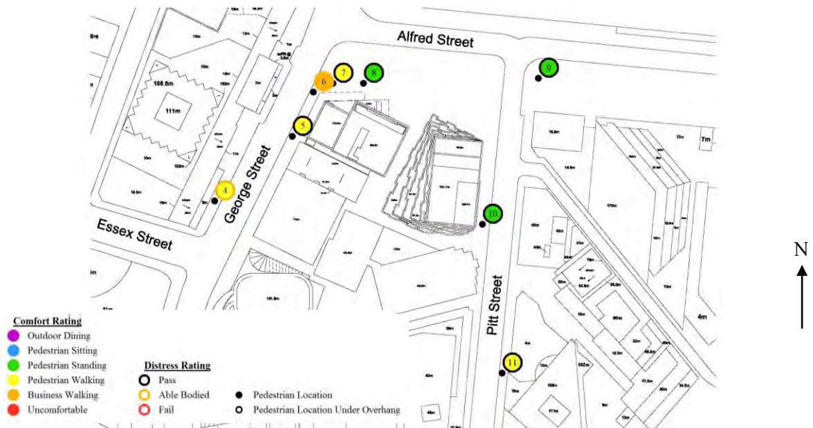
Figure 8: Pedestrian wind speed measurement locations with comfort/distress ratings – Configuration A surrounding locations
