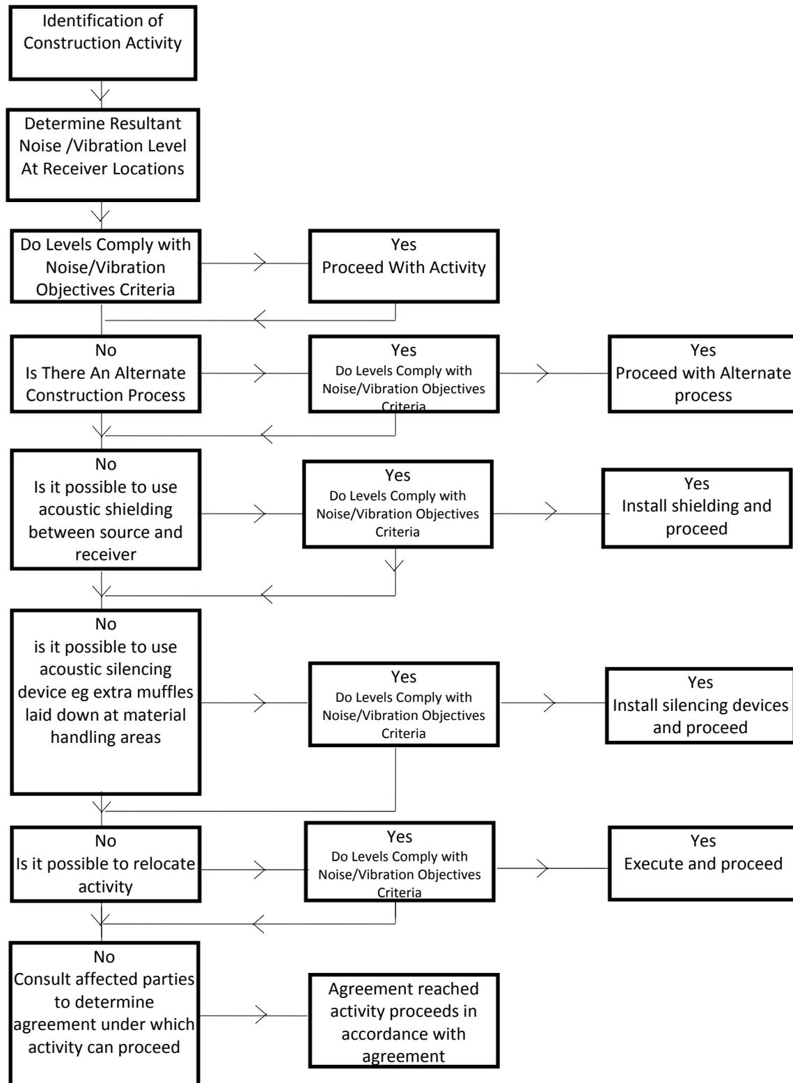
**Figure 2 – Process Flowchart**
