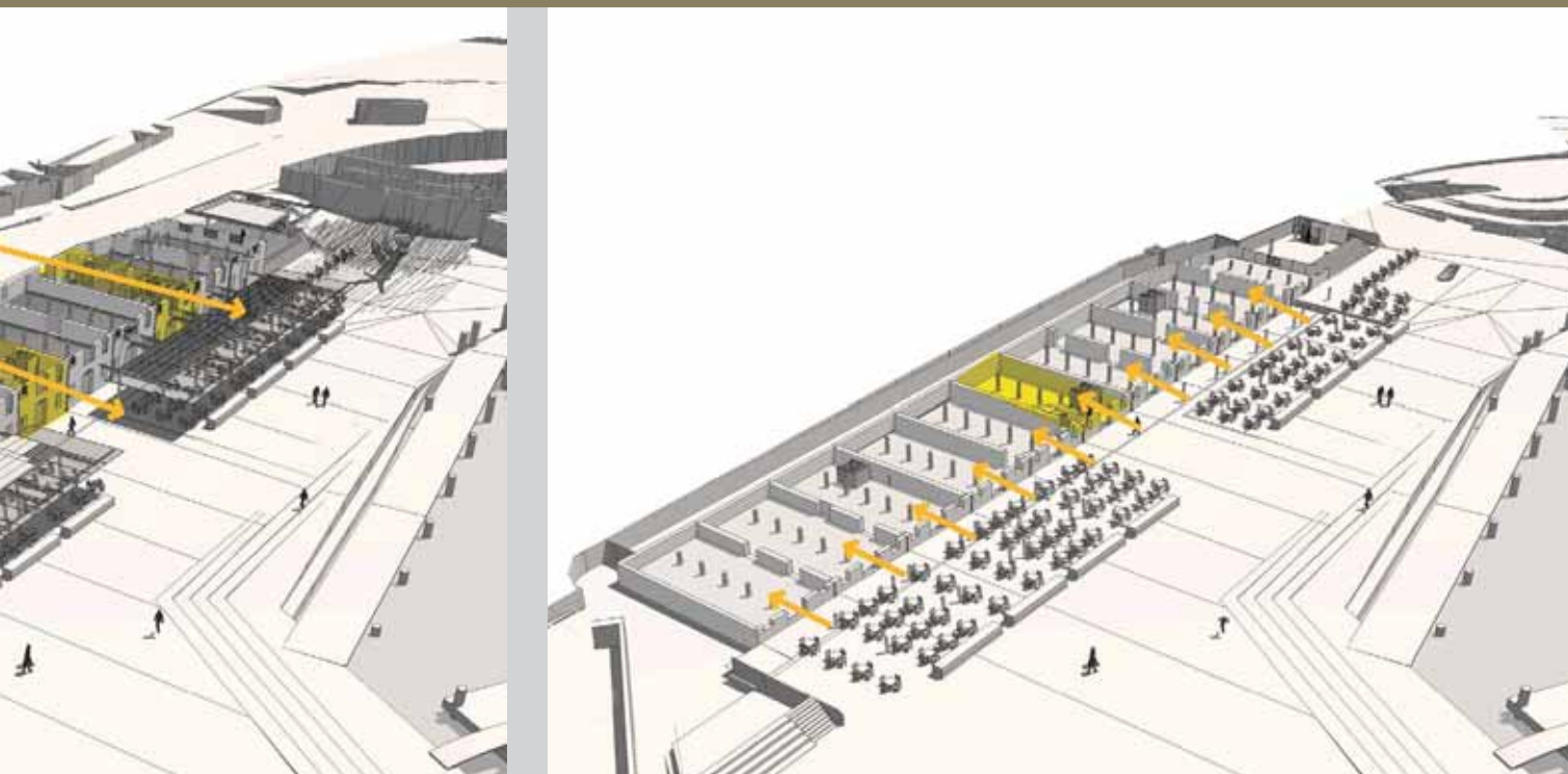
CONCEPTUAL DIAGRAM - GROUND Ground level Natural Ventilation opportunities through existing openings
