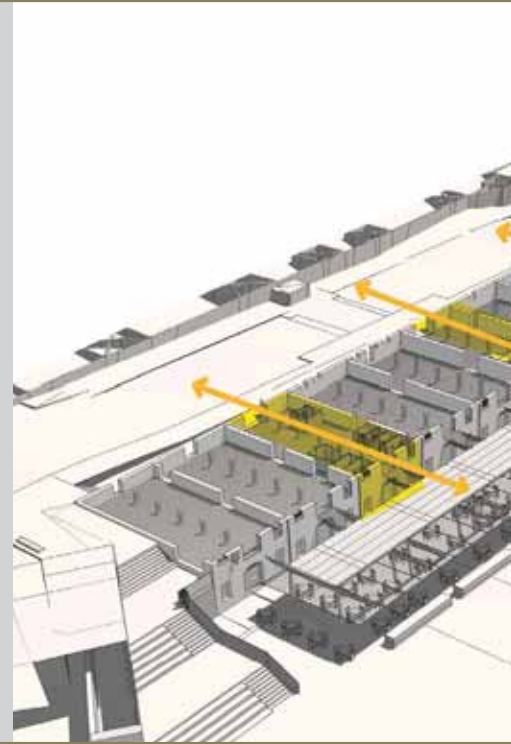
CONCEPTUAL DIAGRAM - LEVEL 1-2 Natural Ventilation cross-flow ventilation opportunities through existing openings & Public Bays
