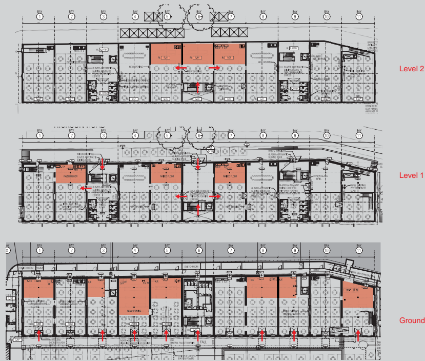
CONCEPT DIAGRAM: Northrop Engineering diagram showing use of existing openings to pull kitchen air exhaust into building.
