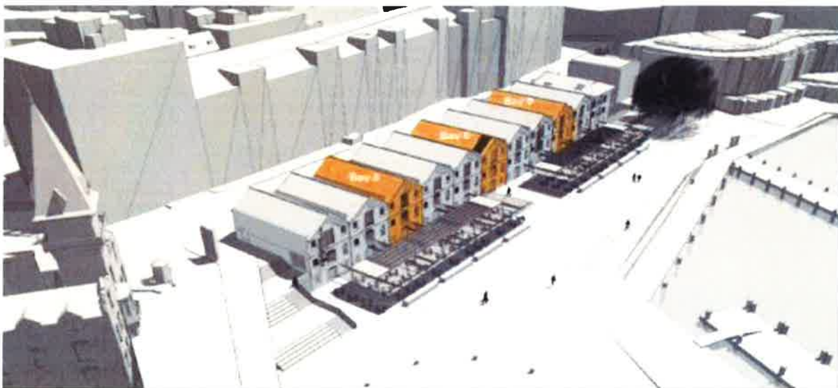
Figure 12: Bays 3, 6 and 9 shown in orange that will accommodate the proposed centralised services including internal lifts, stairs and toilets (Source: Applicant's EIS).
