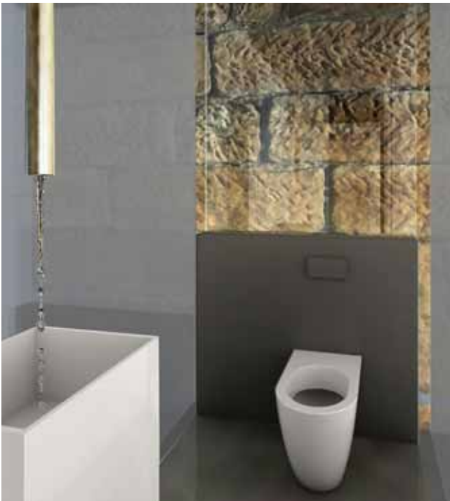
CONCEPT SKETCH RENDERING: Servicing for the toilets will be via a raised floor, and dado walls to take the cistern and equipment.
