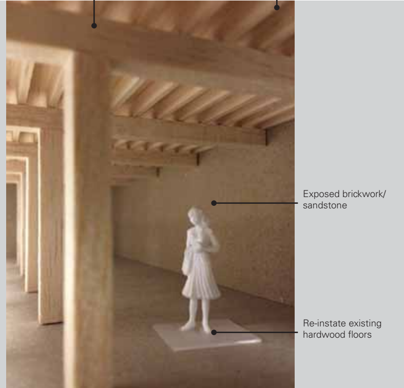
Figure 4.8.4 Interior model photograph showing 'stripped back' tenancy space with heritage structure, soffits, floor and wall revealed
