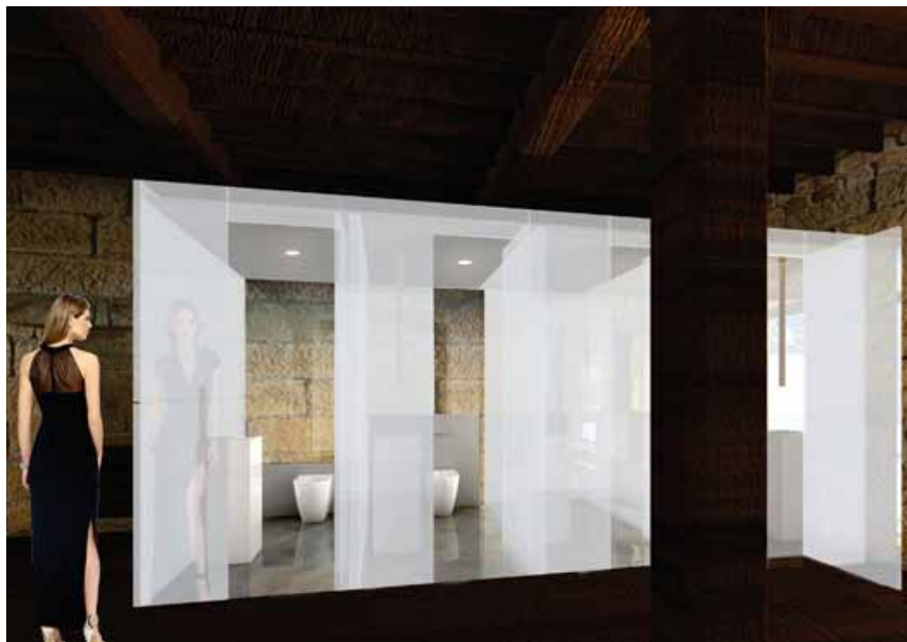
CONCEPT SKETCH RENDERING: The 'boxes' will be of frameless and frosted glass construction, sitting free of the existing heritage structure.
