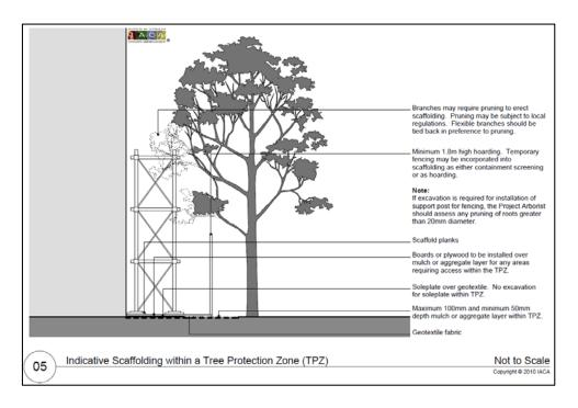
The proposed scaffolding will project approximately 2.0m from the final edge of the building façade, extend from Ground Level to the underside of Level 5; above this level proprietary screens will be utilised which are supported on the as constructed slab edge (not ground
