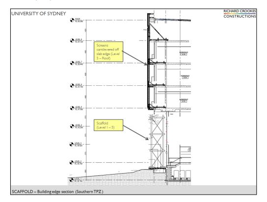
Excerpt photo of screen edge protection proposed for Level 5-Roof as follows:
