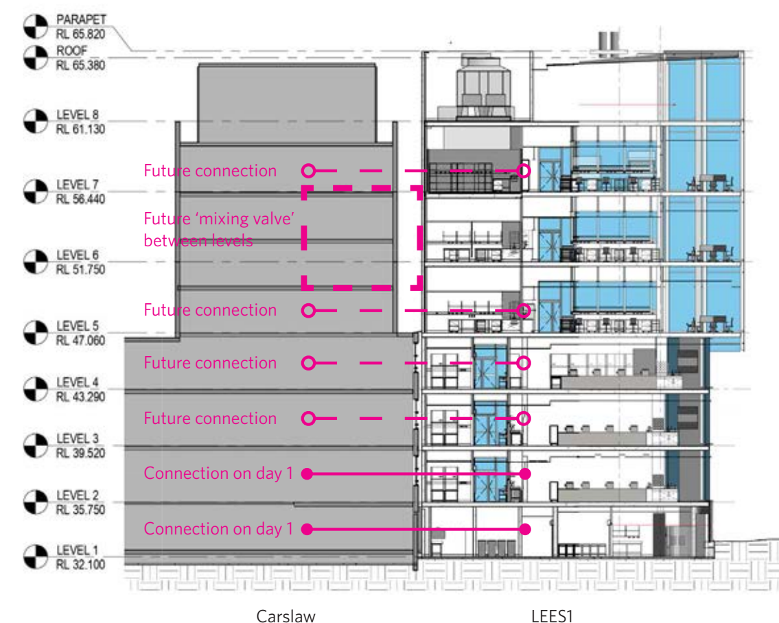
Diagram 1: Section indicating planned functional connections between
