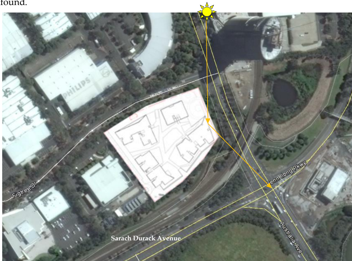
Figure 3: Incident and reflection of solar rays emanating from the East Tower
