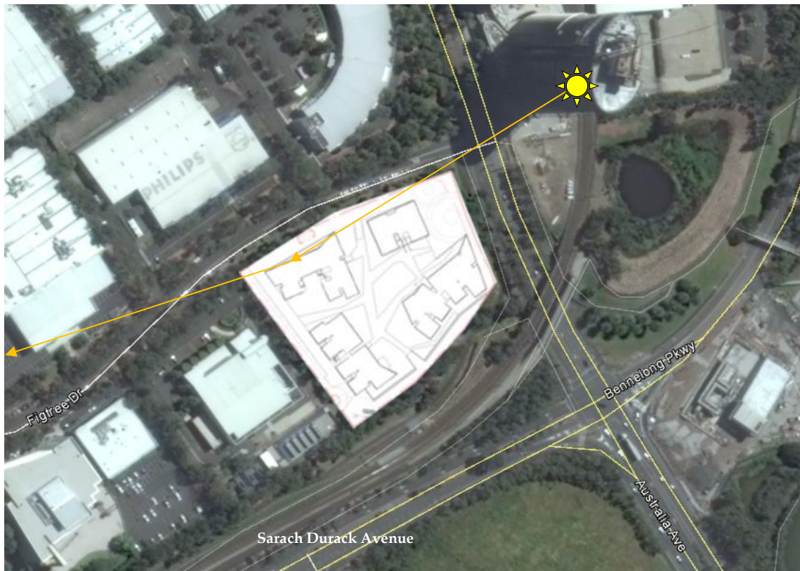
Figure 4: Incident and reflection of solar rays emanating from the West Tower
