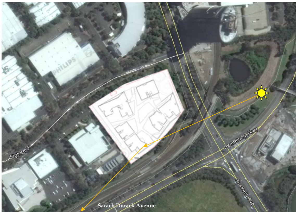
Figure 5: Incident and reflection of solar rays emanating from the South Tower
