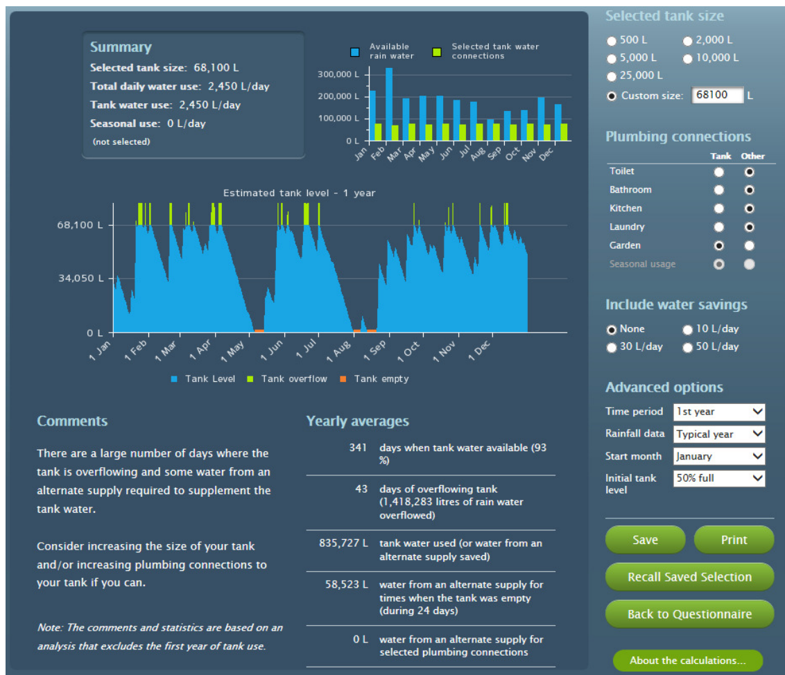
Figure 4 – Roof water harvesting results summary from Tankulator software
