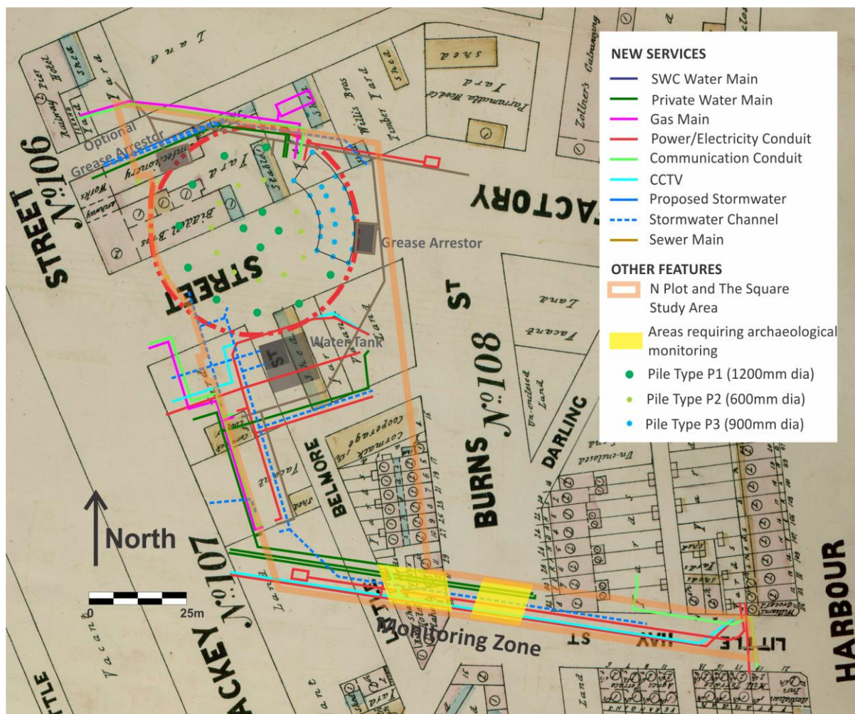
Figure 2: Overlay of impacts (see key) within the North Plot and The Square study area (outlined in orange) onto 1880 historic plan. Note the overlay suggests the services along Little Hay Street will not impact the pre-1880 house on the corner of Burns and Little Hay Streets but will have some limited impacts on the c.1815 Dam Wall. Base plan Dove 1880.
