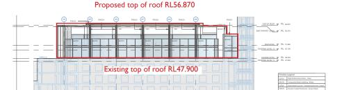
Figure 6. West Elevation of the SSD-7014 proposed executive bar and business centre (Courtesy of COX Richardson)
