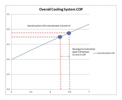
As Basix only recognizes overall system COP's up to 4.5, it would be required that an algorithm is entered into the calculations which allows for higher COP's.
