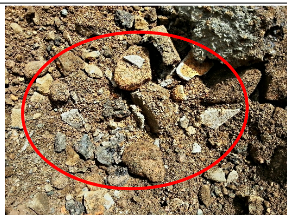
Photo 3. Stockpile 225, Excavation Area – Presumed asbestos-containing fibre cement fragments
