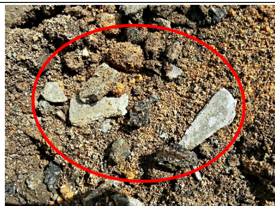
Photo 5. Stockpile 225, Excavation Area – Presumed asbestos-containing fibre cement fragments
