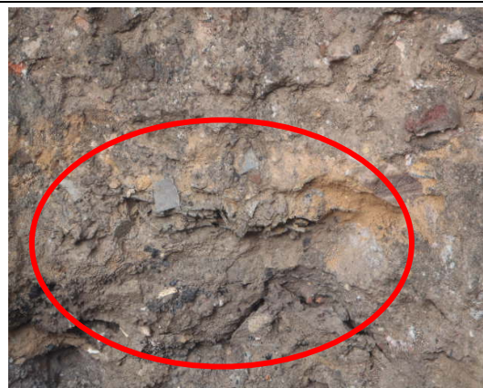
Photo 18. Stockpile 225, Excavation Area – Presumed asbestos-containing fibre cement fragments
