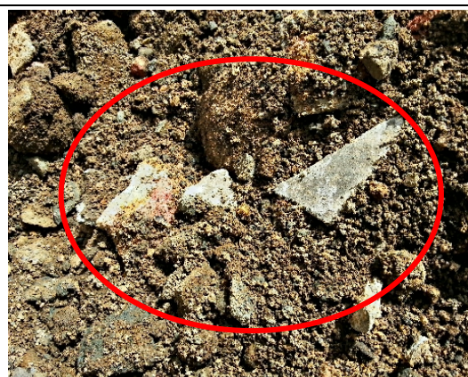
Photo 4. Stockpile 225, Excavation Area – Presumed asbestos-containing fibre cement fragments
