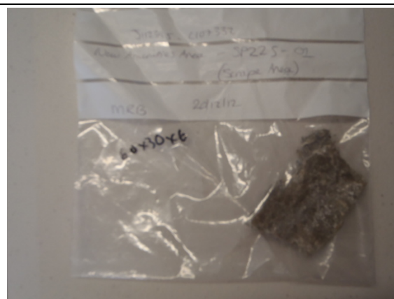
Photo 1. Stockpile 225, Stockpile Area – Confirmed asbestos-containing fibre cement fragment
