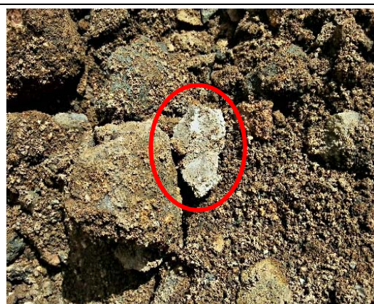
Photo 2. Stockpile 225, Excavation Area – Presumed asbestos-containing fibre cement fragment
