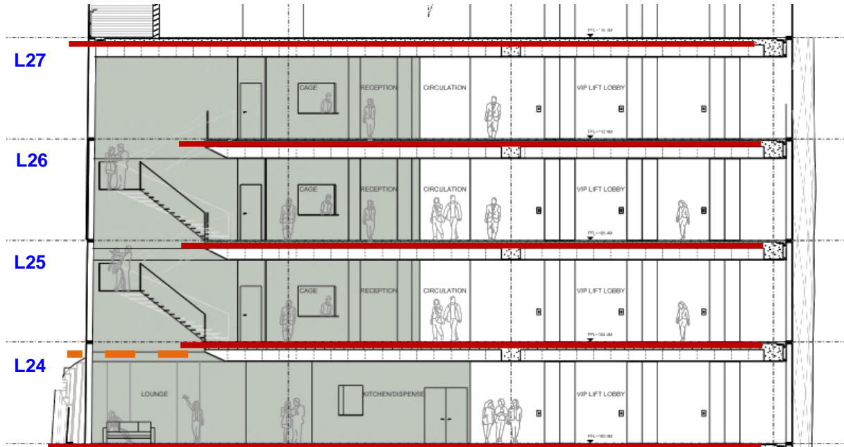
Figure 5-19: Section through the Crystal club and the sky gaming levels with orange dashed line indicating location of proposed horizontal fire curtain.
