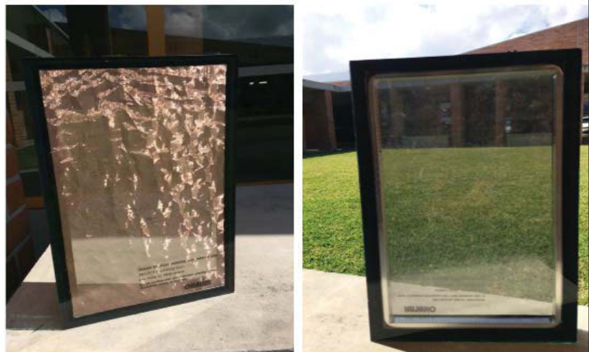
IGU WITH SUN CONTROL METALLIC INTERLAYER
