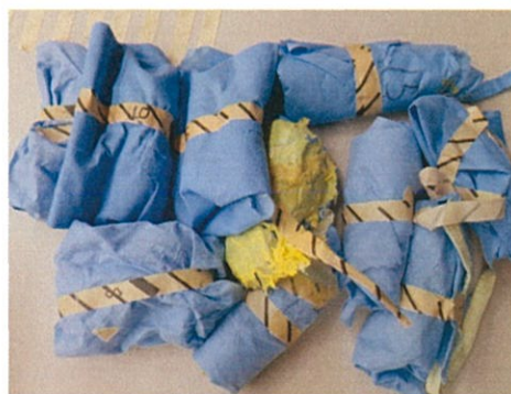
Figure 3: example of the wrapped BI's with autoclave tape
