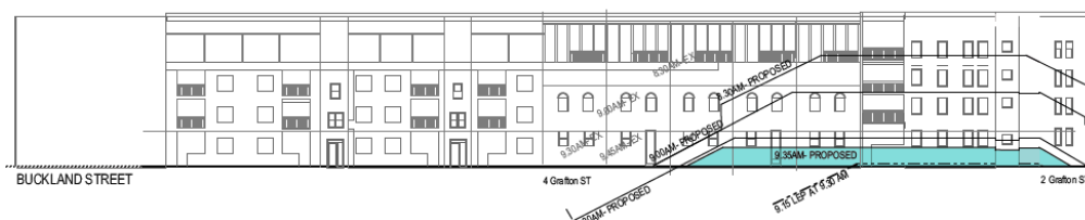
Figure 2 Extract from solar elevation diagram, showing that there is no midwinter overshadowing of any residential windows after 9.35am
