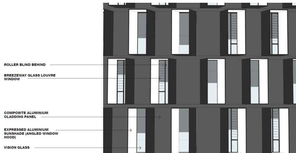
Figure 3 – Detail of angled window hoods
