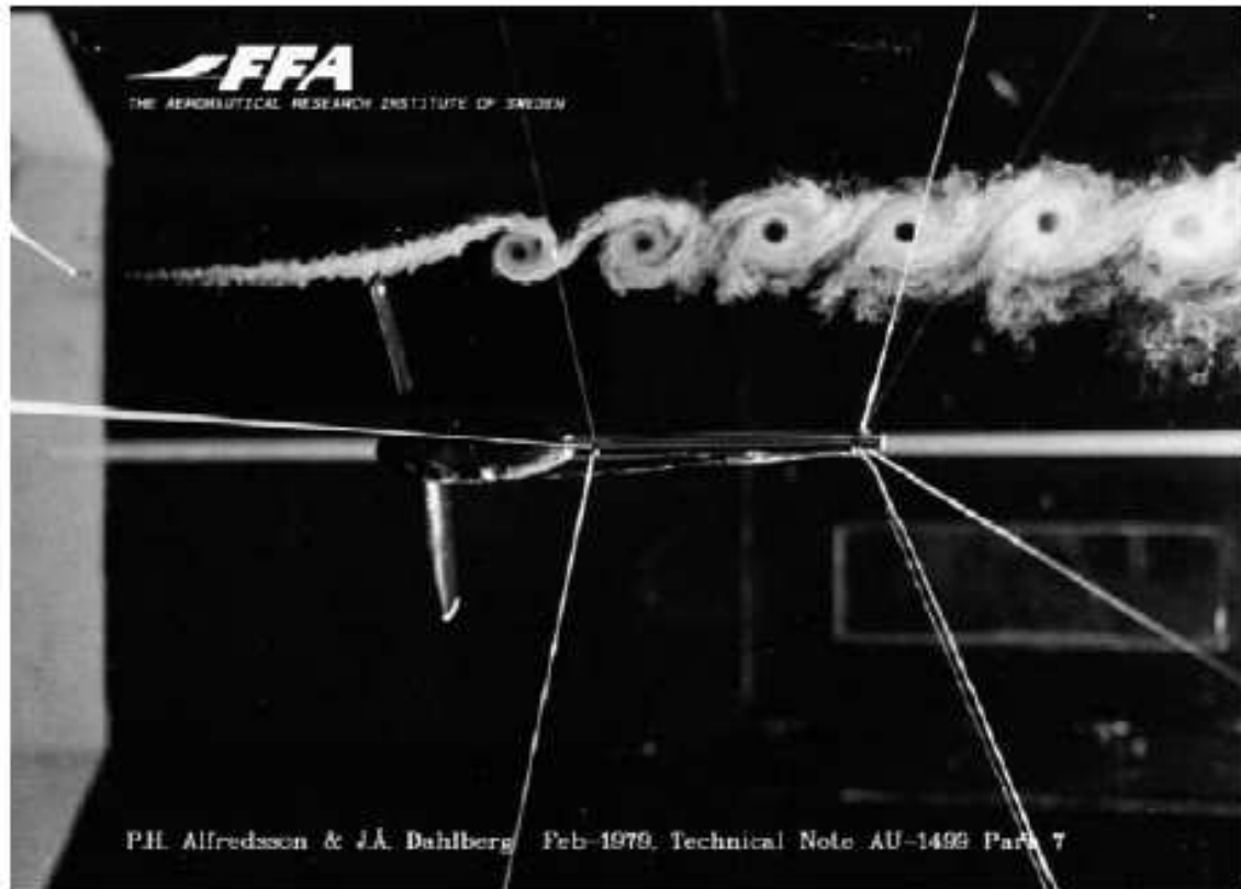
Figure 1. Smoke trail passed over blade-tips showing vortices [Ref 1]
