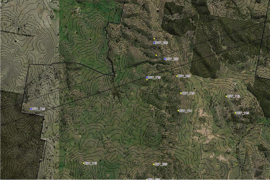
Figure 4-3 – Zoomed-in aerial showing radio-communications link from left to right and turbine locations within this Fresnel zone in blue.
