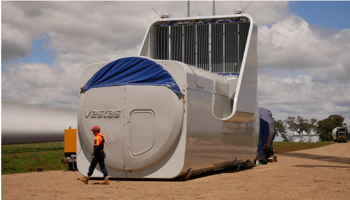
Figure 1-12: Example of a nacelle for a 3.6 MW WTG at Sapphire Wind Farm
