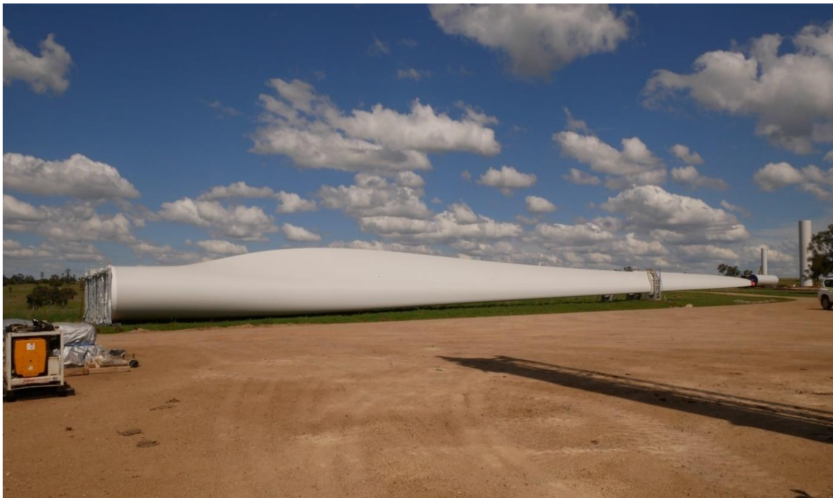
Figure 1-13: A single piece blade approximately 62 m long at Sapphire Wind Farm
