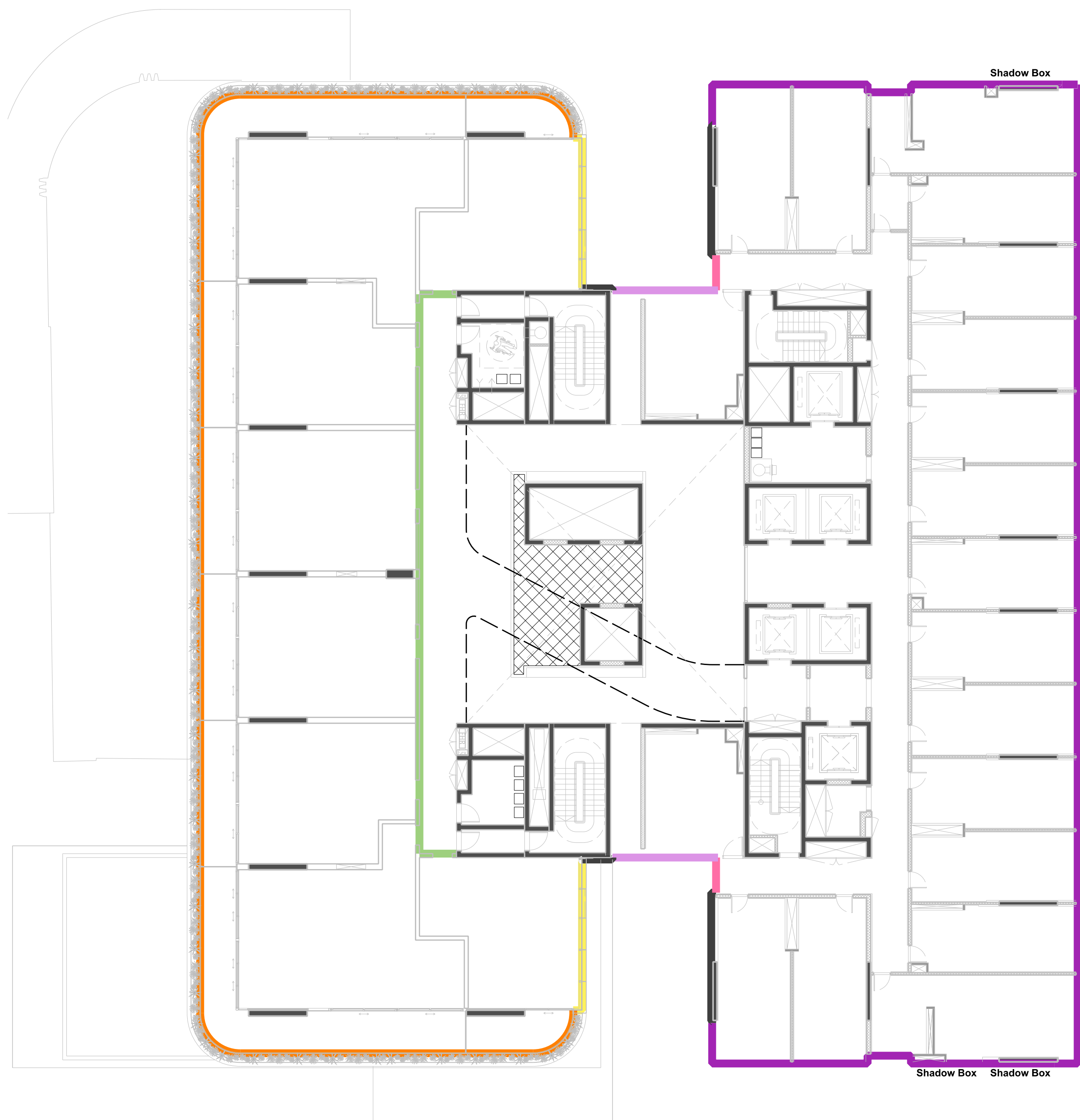
03 Cladding Typologies - Plan Resi (L11) / Hotel (L13) 1:20
