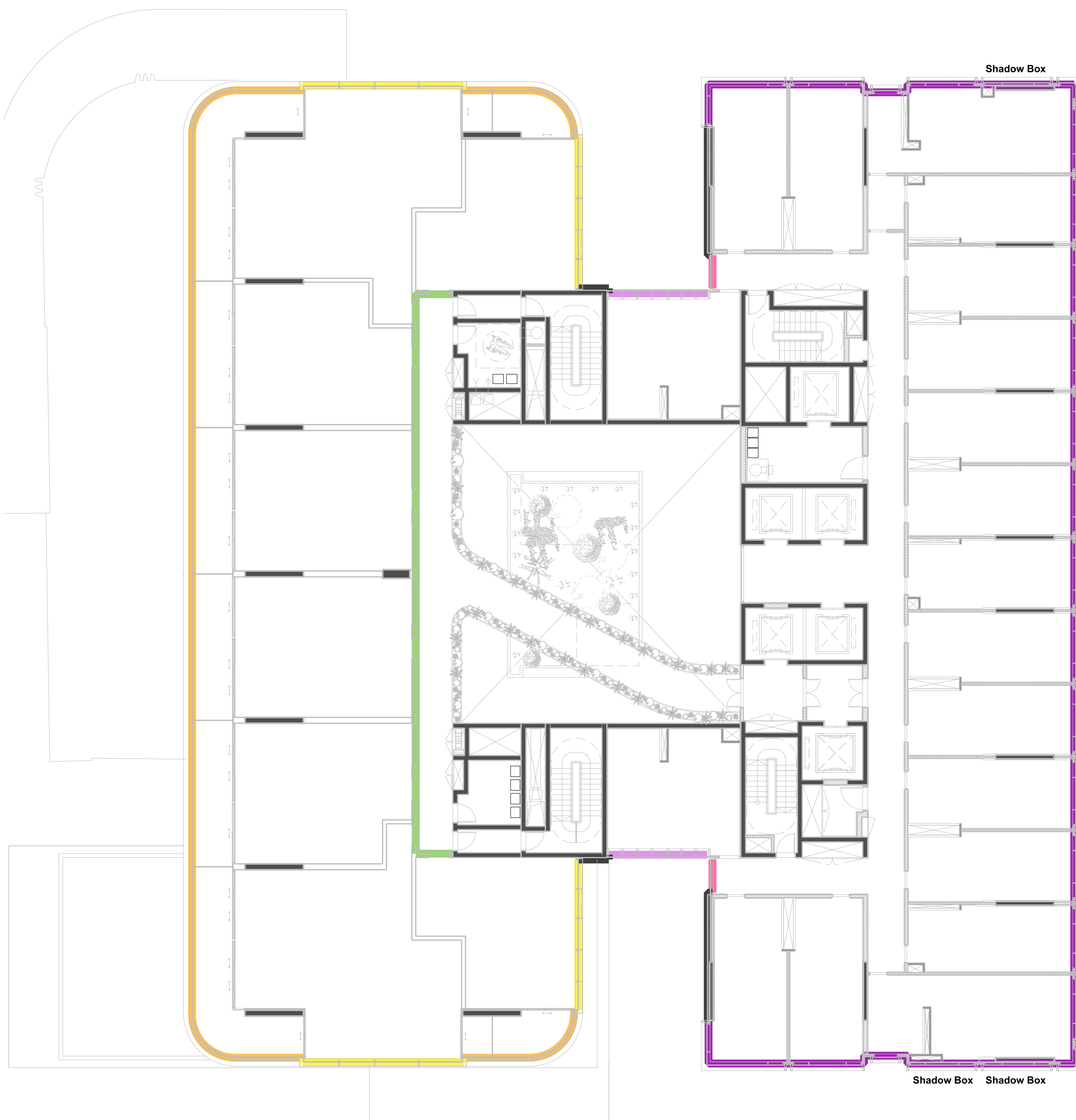
04 Cladding Typologies - Plan Resi (L12-16) / Hotel (L14-18) 1:20
