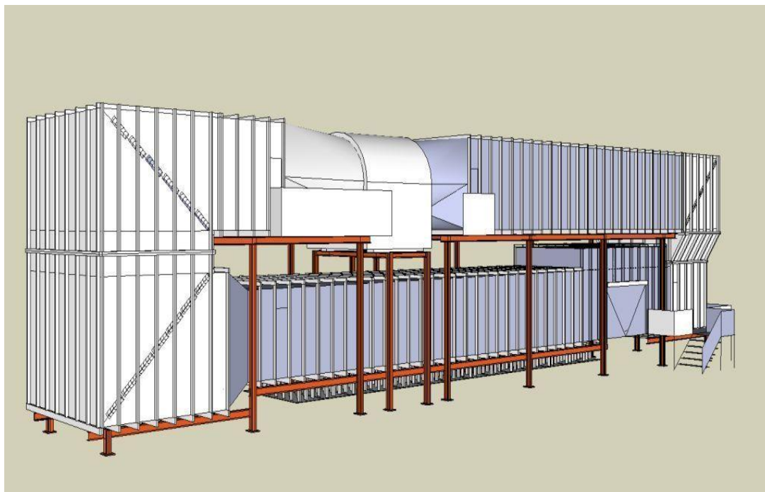
Figure 3: Schematic of the closed circuit wind tunnel
