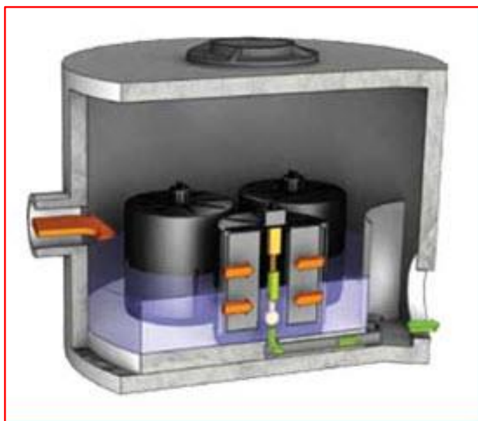
Figure 9: Filtration of Stormwater Pollutants in a StormFilter System (Source: Stormwater360)
