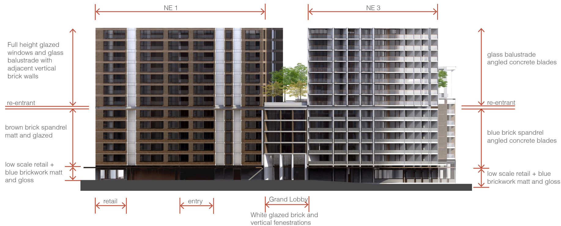
Figure 7.4 – Podium East Elevation facade and materiality
