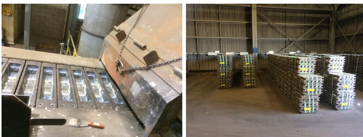
Figure 3-8: Ingot mould conveyor (left) and stored ingot awaiting transport (right)
