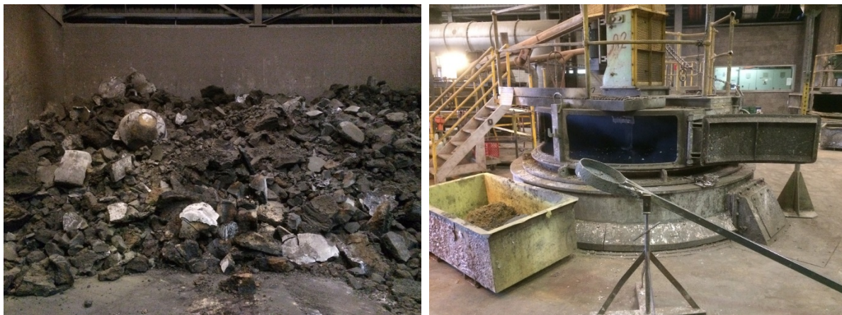
Figure 3-7: Slag or naturally immobilised waste (left) and a refining kettle (right) with dross ladle and bin.
