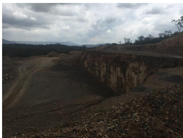
Photo 6: Northern face (Bench 2). Tension cracks in overburden (soil) material visible.
