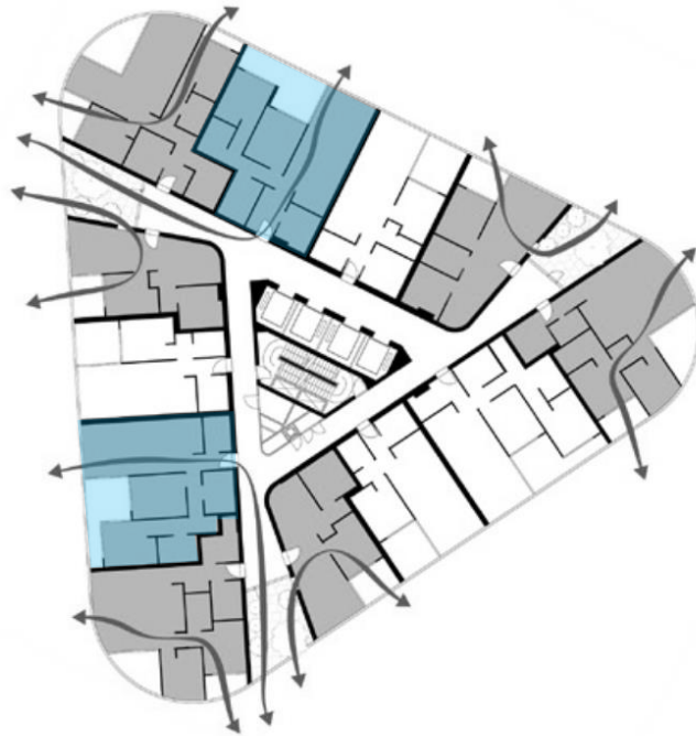
Figure 1 Cross-ventilation apartments; dual aspect (grey) and via plenum (blue)
