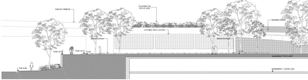
DETAILED ELEVATION OF INTAKE VENT SCALE 1:200 @ A3
