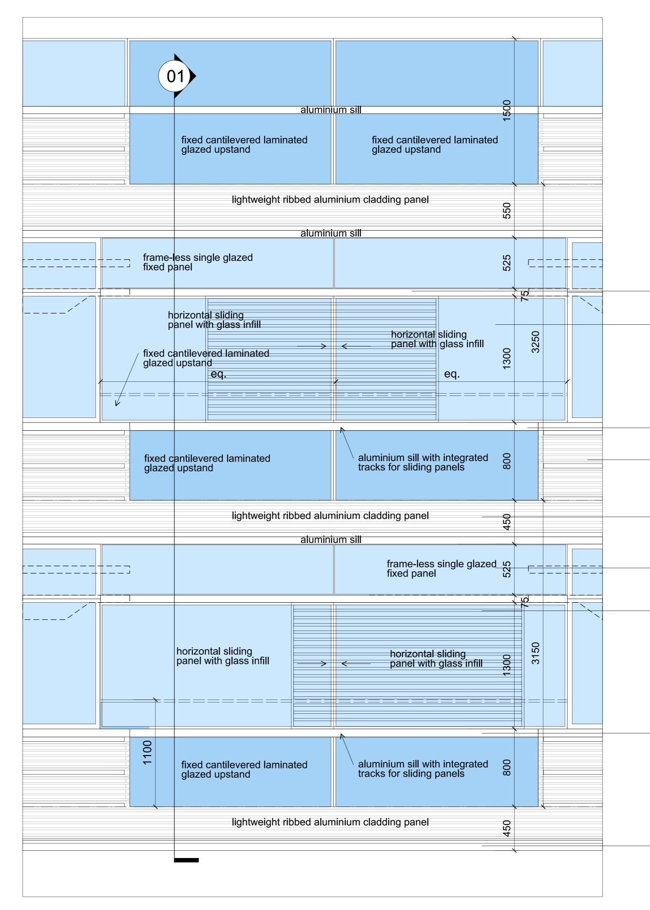
02 Cladding Type C - Typical Loggia Facade - Elevation
