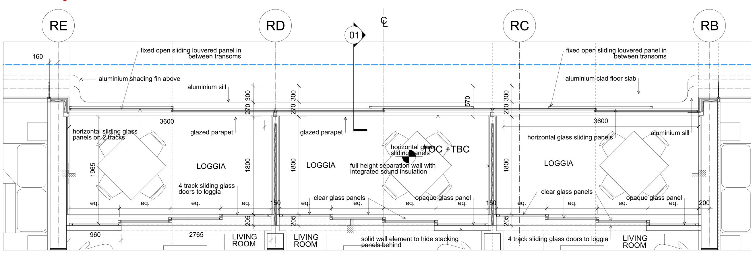
03 Cladding Type C - Typical Loggia Facade - Plan
