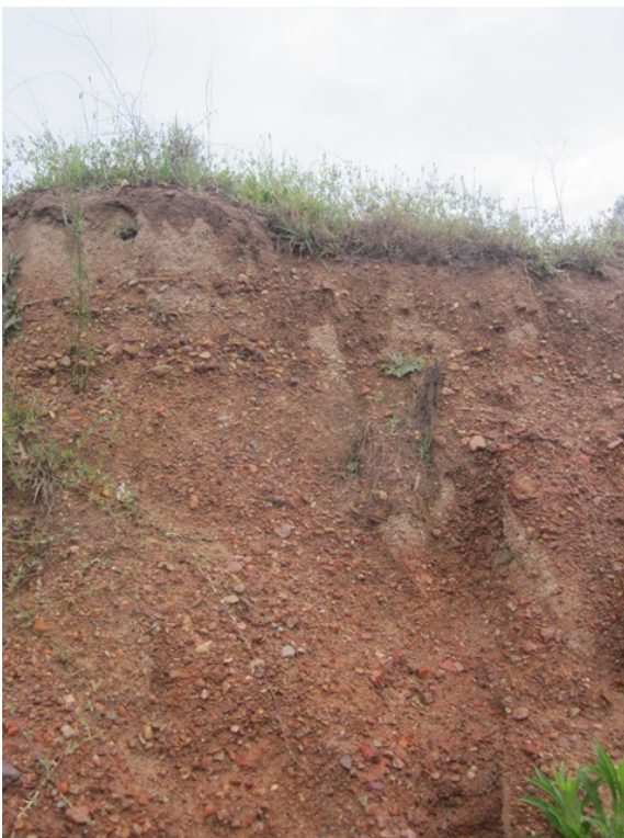
Plate 5 Colluvial gravel, B and C horizon material in the quarry area. The photo shows accumulated gravel in a sandy clay matrix, and two lag deposits
