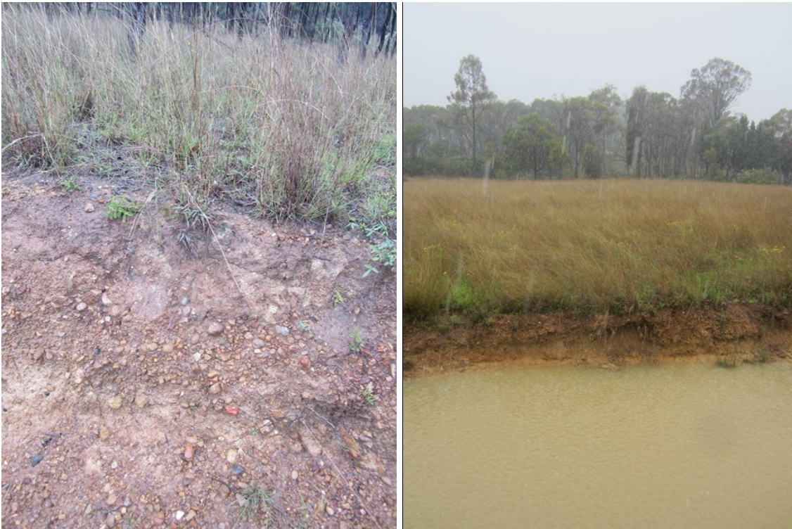
Plate 6 and Plate 7 Profile developed on upper slope bench in the proposed quarry area. Conglomerate cliffs are located upslope, approximately 150m away. These photos show a partially stripped A1 horizon, a strong concentration of gravel in the lower A2 horizon, bleaching in the A2 horizon, mottling in the upper B horizon (sandy clay) and poor drainage
