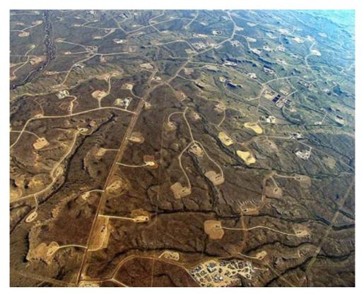
Figure 5: Dense well spacing in the U.S. state of Wyoming http://www.sacurrent.com/sanantonio/the-shale-booms-hard-sell-begins-pushing-up-against-reality/Content?oid=2341996
