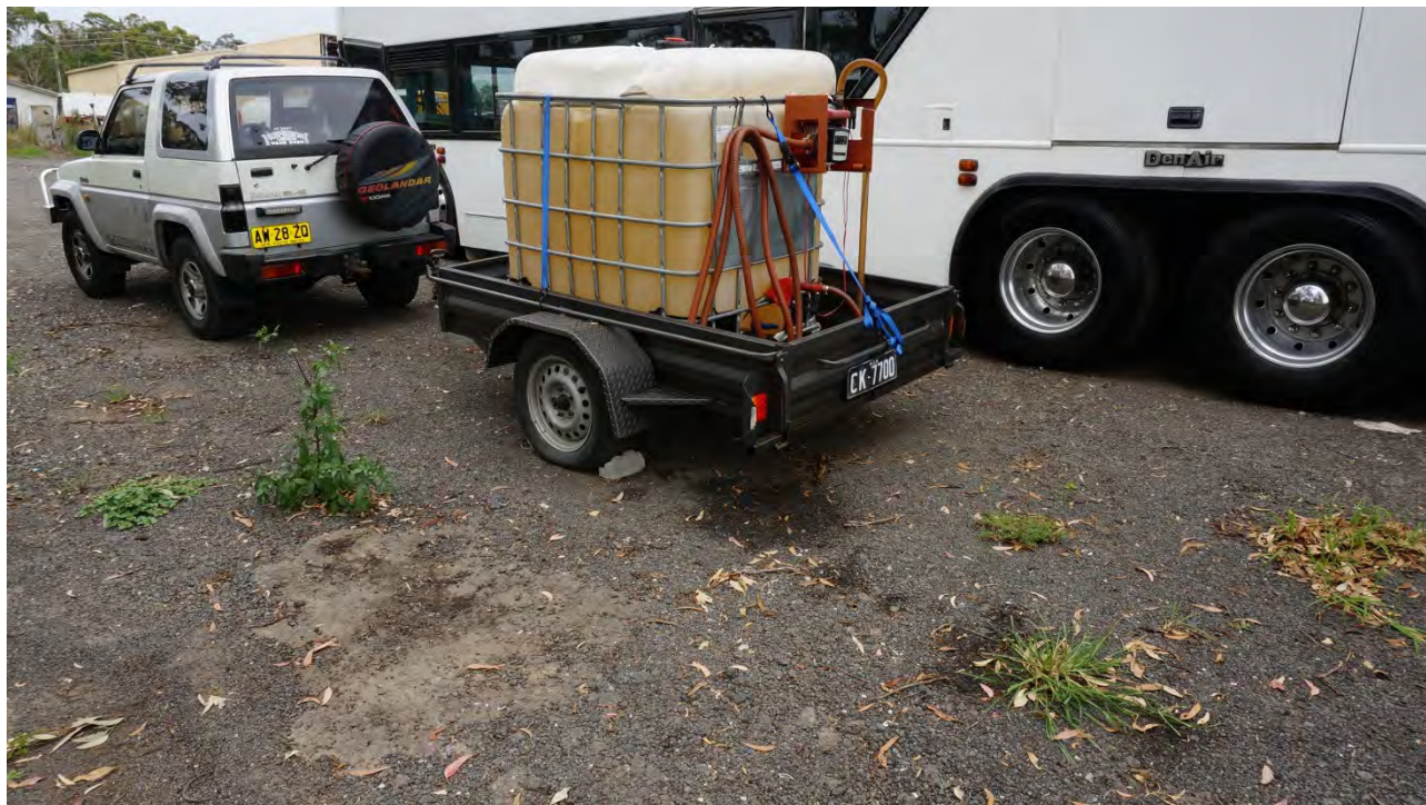
31 Trailer mounted IBC used to dispense diesel. Note hydrocarbon staining below trailer.
