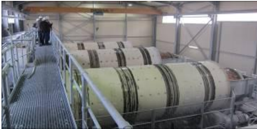
Figure 6: Washing kaolin from silica sand in trommel drums at Quarzwerke Hirschau plant
