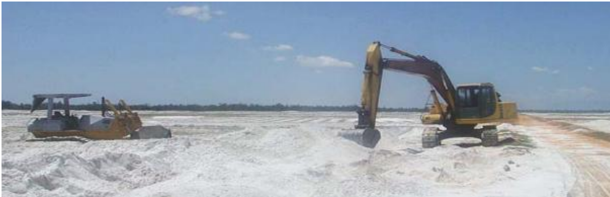
Figure 4 Typical silica sand mining 60 km south of Danang Vietnam. Bulldoze then load truck Sand depth ~ 2 metres.
