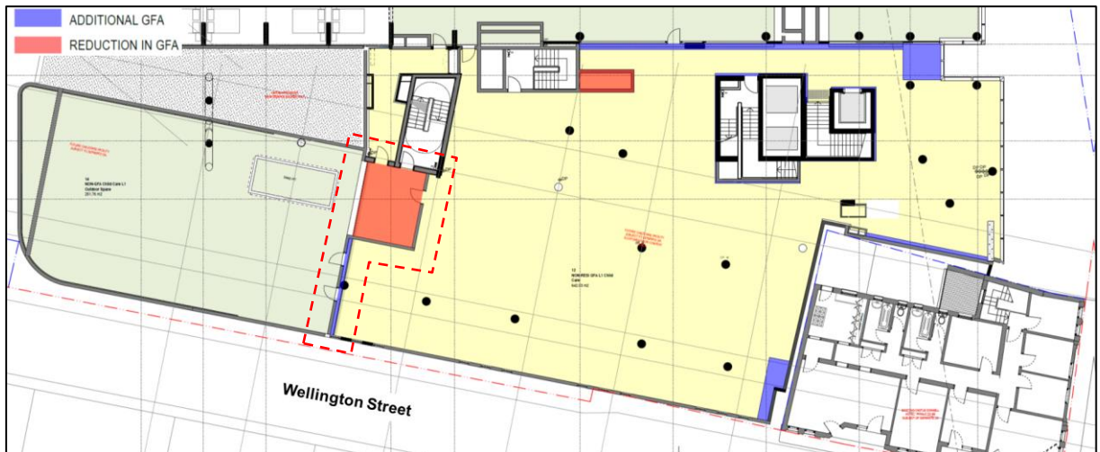
Figure 7: Revisions to childcare centre façade line (bordered in red) and corresponding change to non-residential GFA (Source: Applicant's EIS)
