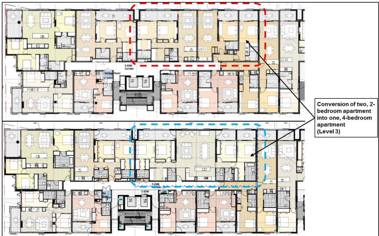
Figure 4: Approved (top) and modified (bottom) Level 3 layout, including the creation of a 4-bedroom apartment (Base source: Applicant's EIS)
