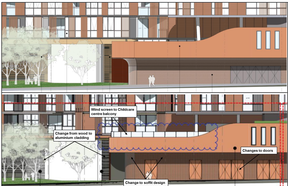
Figure 5: Approved (top) and modified (bottom) southern elevation fronting Wellington Street (Base source: Applicant's EIS)
