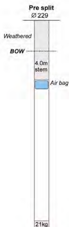
Figure 12 – Indicative pre split blast hole loading
