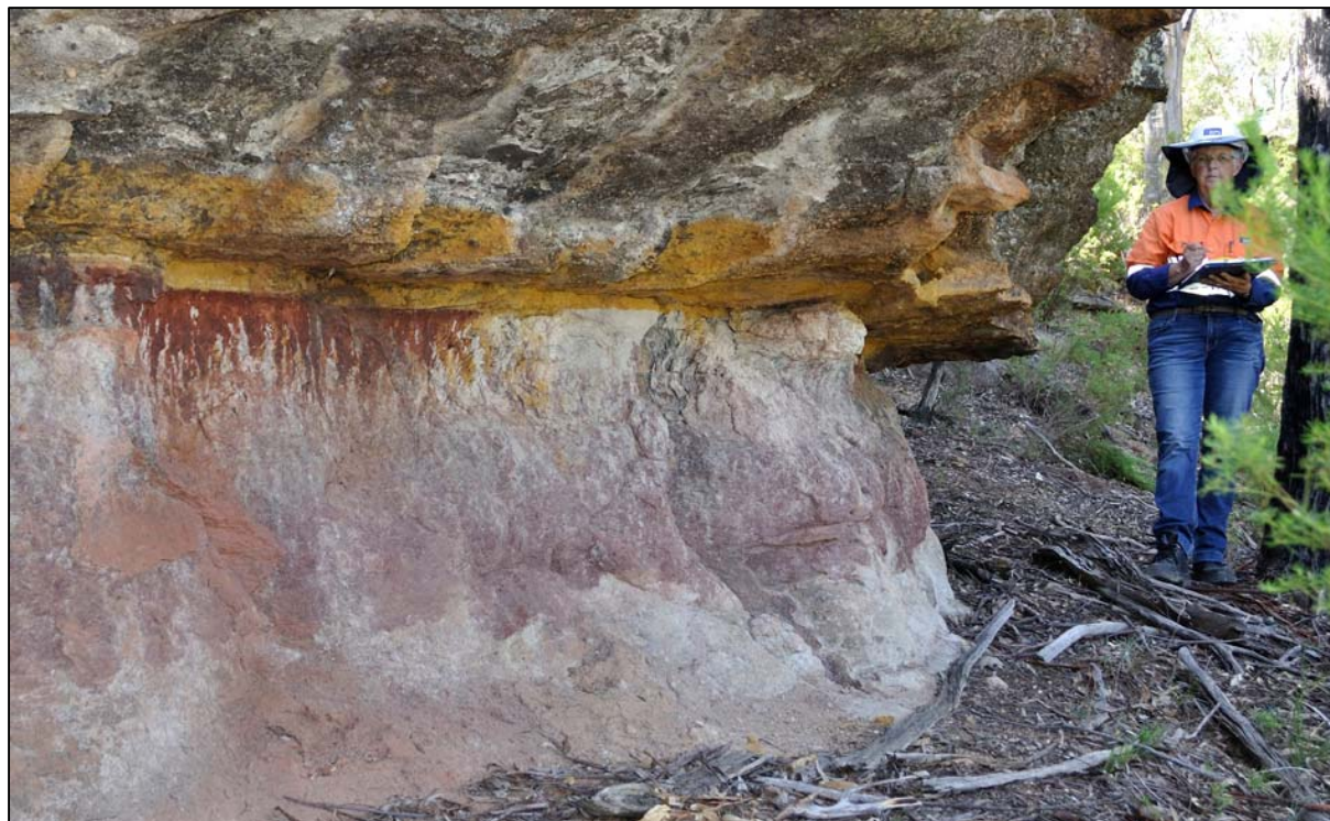
FIGURE 7: Upper yellow ochre layer above the mottled red and grey sandy-clay with red 'bleeding' from below the yellow layer
