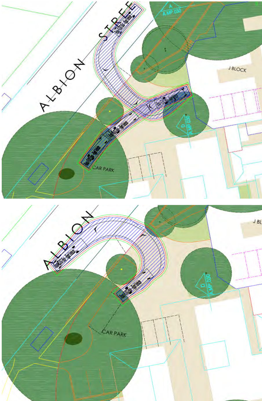
Figure 30: Swept path of FUSO minibus at Gate 1
