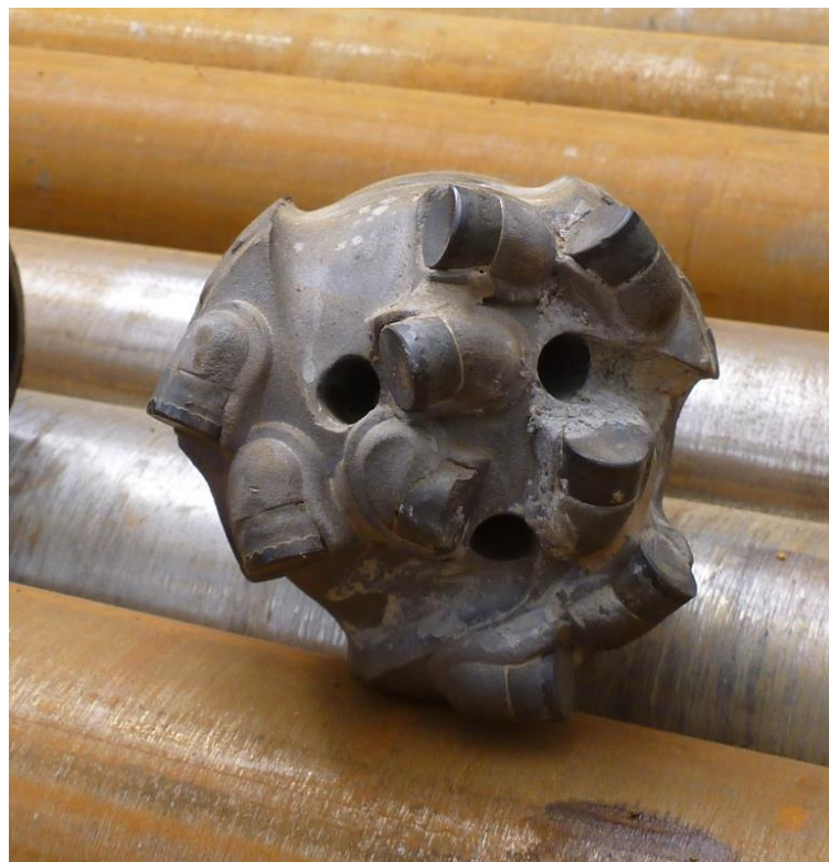
Photograph 2 PCD button bit used for open hole drilling at Sutton Forest
