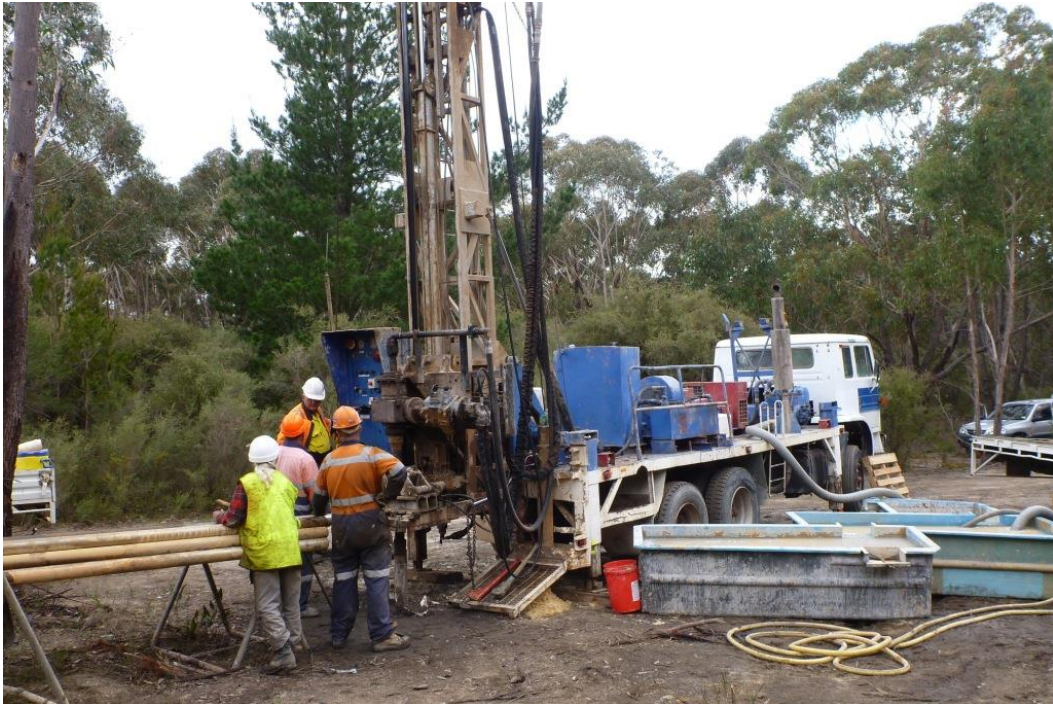
Photograph 1 Pioneer Mole rig during diamond core drilling at Sutton Forest
