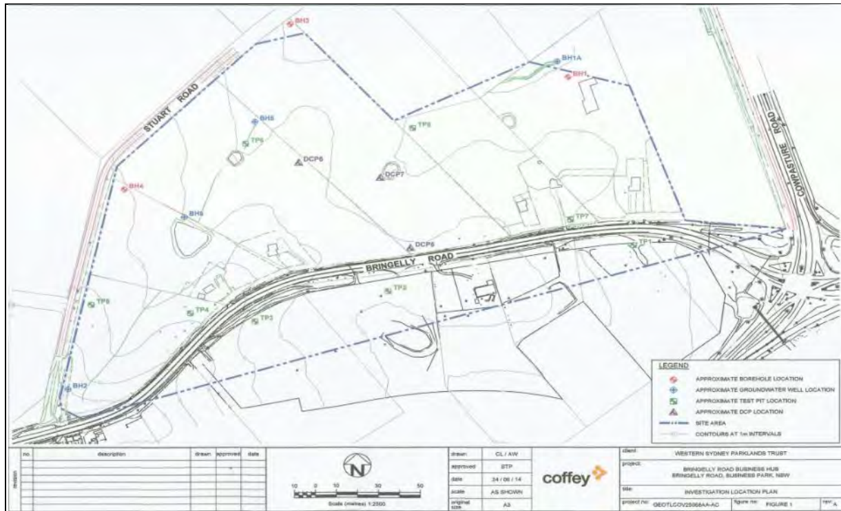
Figure 1.2: Survey plan and geotech borehole location (Source: Coffey 2014)
