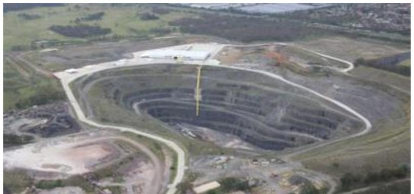
**Image 1 Genesis landfill showing chute from Material Processing Facility**
