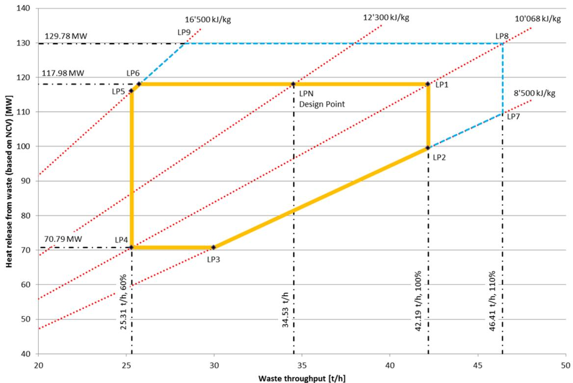
Figure 5 Combustion diagram for 1 Line
