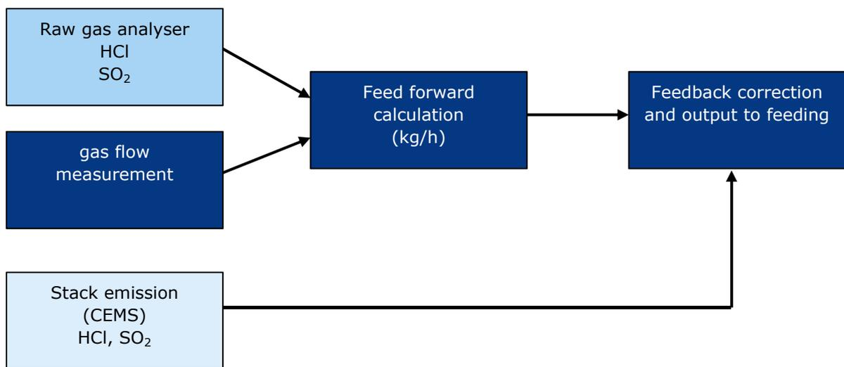
In case of a malfunction of the raw gas analyser, the operator can either run the plant with a default value for the raw gas concentration (e.g. the observed average) or without the feedforward part of the control logic (just using the feedback controllers). With this setup the emissions are maintained below the required limits, but there might be slightly higher lime consumption.
