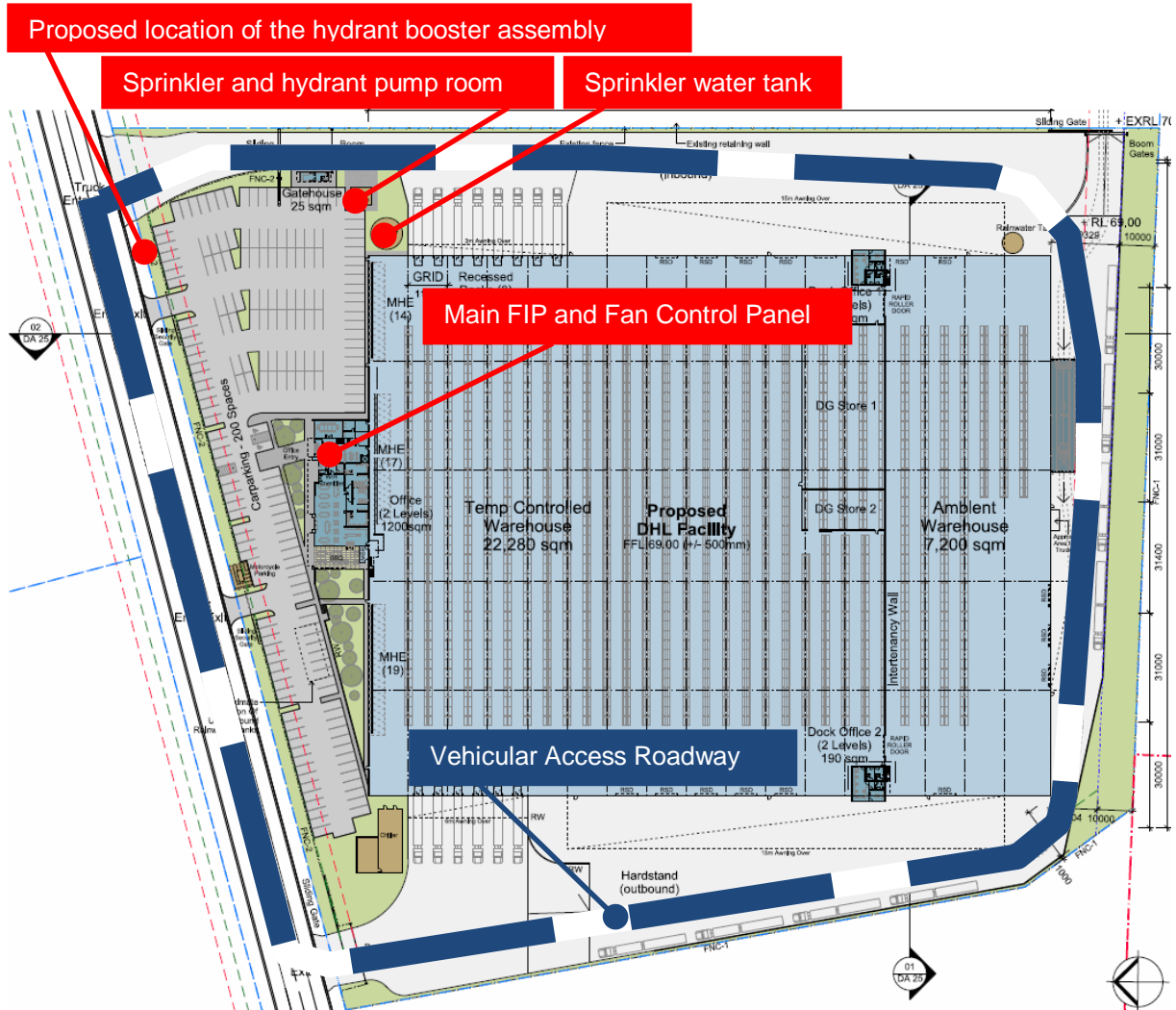
Figure 7-3: Site plan illustrating the location of fire services and fire brigade access roadway
