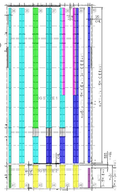
Plan 3-2 Proposed Dangerous Goods Storage Location Source: Figure 3-2 (page 12) PHA Report. Note: Refer to Warehouse Racking Layout Plan for DG storage measurements
