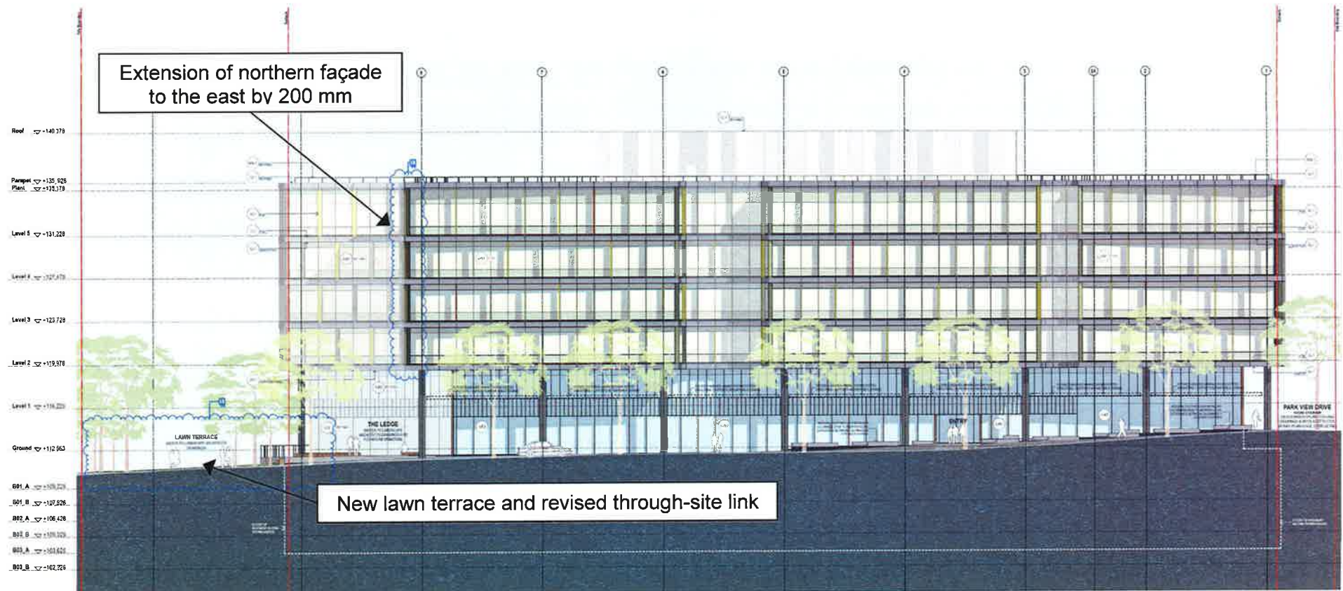
Figure 5: Modified northern elevation of commercial building
