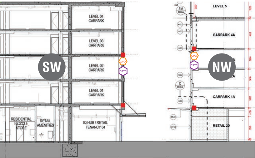
Indicative section of fixing to SW and NW Plots Steam Mill Lane - NTS (Diagram by Event Engineering)
